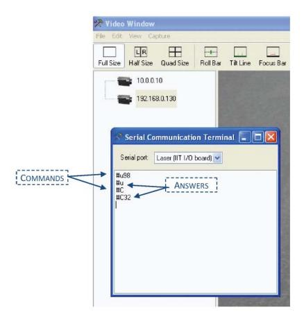
The DAC values in commands C to J are set to 32 from the factory and it is normally not necessary to change these.
